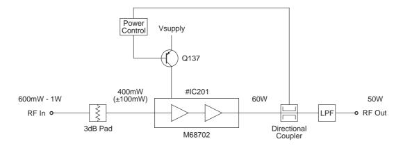
Figure 2.1 T838 High Level Block Diagram
