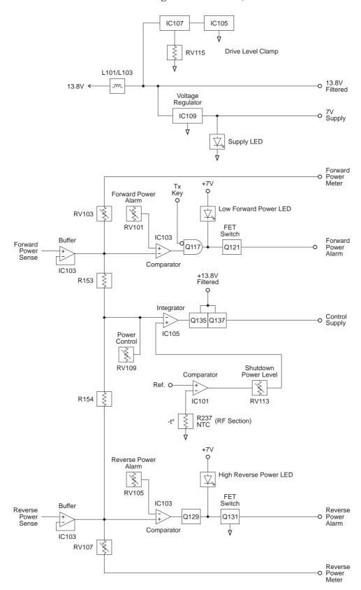
Figure 2.3 T838/839 Control Circuitry Block Diagram
