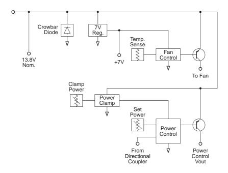
Figure 2.5 T838/839 Power Supply & Regulator Circuitry Block Diagram
