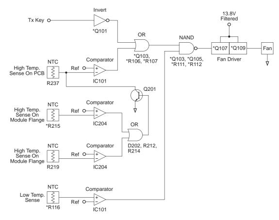
Figure 2.4 T839 Fan Control Logic Diagram
