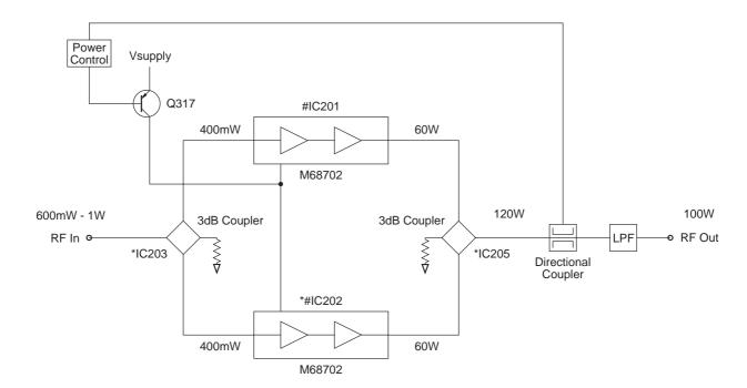
Figure 2.2 T839 High Level Block Diagram
